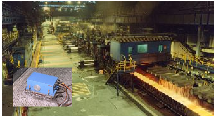
Photograph shows a typical installation of a Landscan sensor head.
